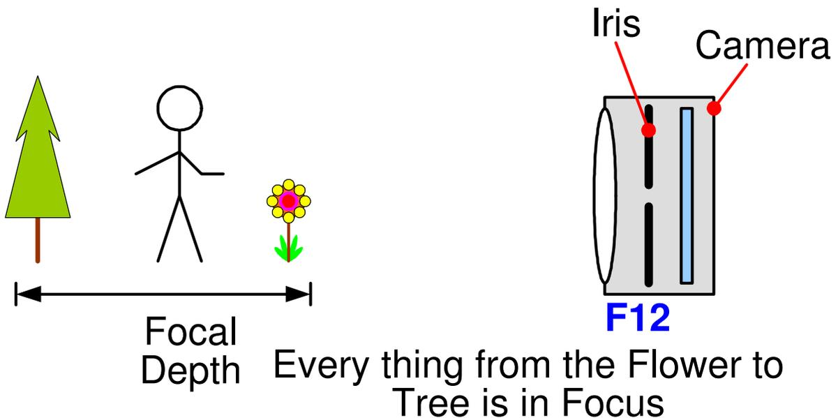
The size of the aperture is giving as a number, and the bigger the number the SMALLER the aperture (smaller hole). It is some time called the 'F' number as it has an 'F' in front. (This is only a basic explanation read more if you want).
